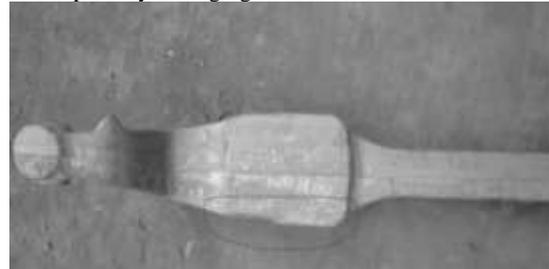
Fig. 7: Underfill pad section of front axle beam
