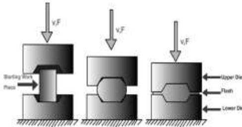
Fig. 2: Stages of closed die forging process
