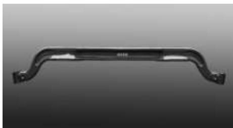
Fig. 5: Front axle beam
