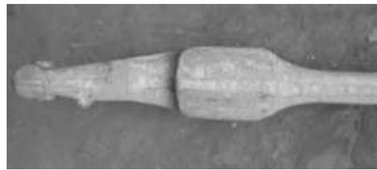
Fig. 6: Completely filled pad section of front axle beam
