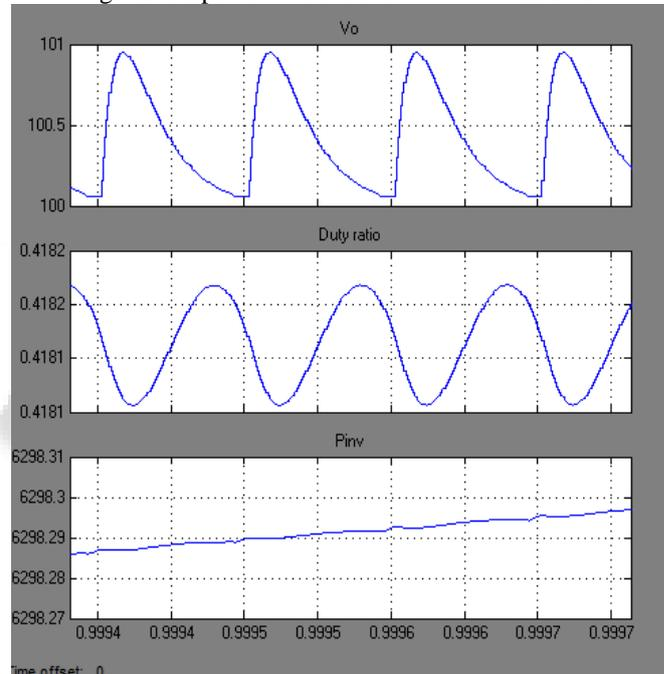
Fig. 14: outputs of PI controller with FF control
