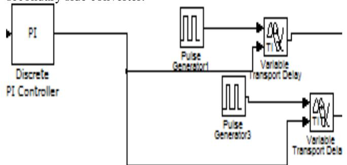
Fig. 3: Delay pulses generation
