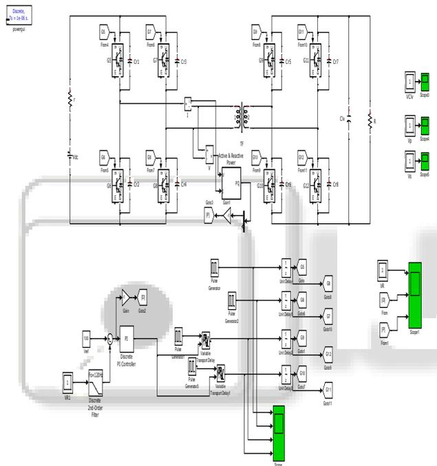
Fig. 11: complete simulink model of DAB
