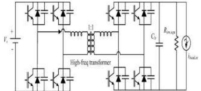
Fig. 1: DAB circuit for PVA application
