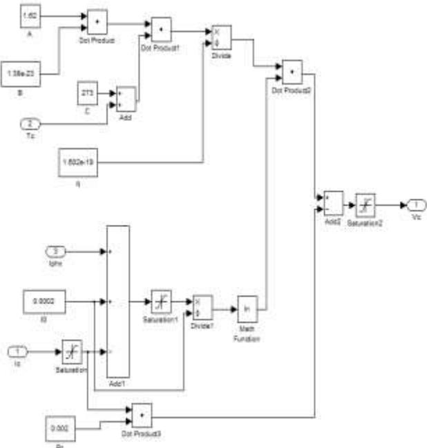
Fig. 6: Simulink model of Vc
