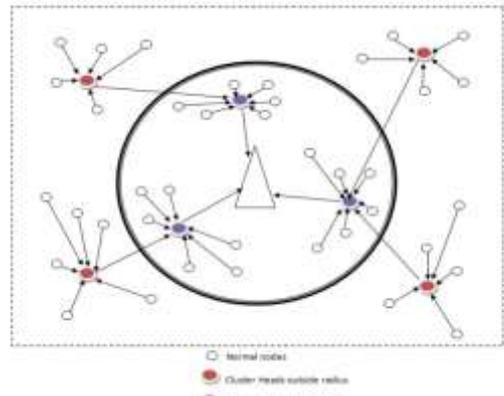
Fig. 4: Minimum Transmission LEACH Protocol Architecture
