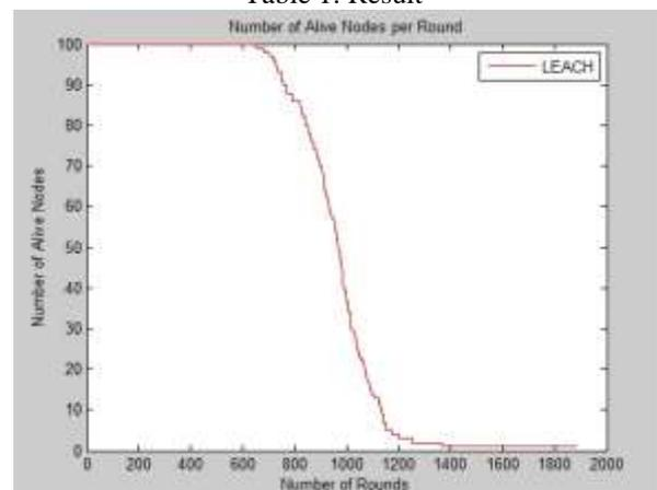
Fig. 5: Simulation Results of LEACH
