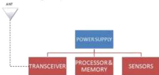
Fig. 1: Sensor Node Architecture
