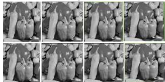
Fig. 11: The first column: Original image; the second column: compressed at q=10 and q=50/3; the third column: obtained through Dic-TV method; the fourth column: Dithering method.
