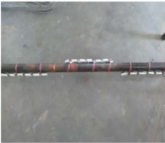
Fig. 4: Short inserts wounded on inner copper tube
