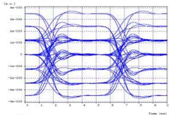
Fig. 5: Received eye diagram for video signal
