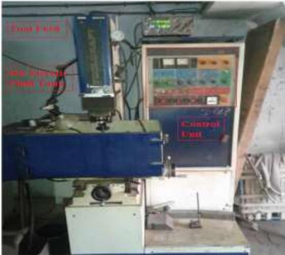
Fig.1 Toolcraft A25 EDM Machine
