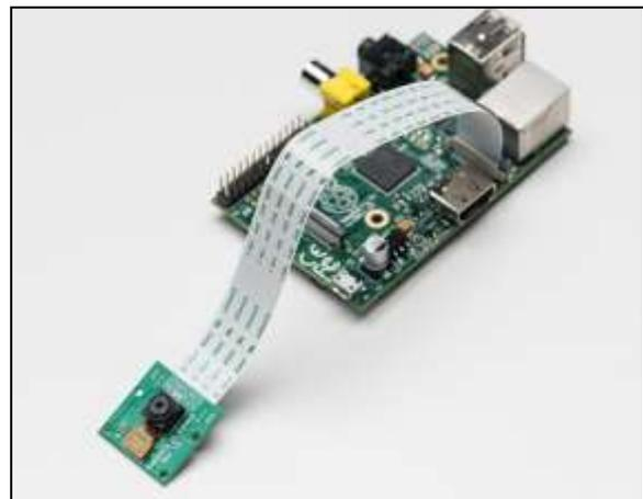
Fig. 7: Raspberry Pi Interfaced With Camera Module
