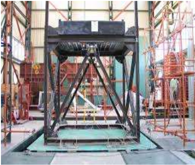
Fig. 3: shows INVERTED V-bracing
