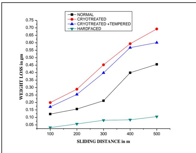
Fig. 6: (C) Graph of Weight Loss in Grams to Sliding Distance in M
