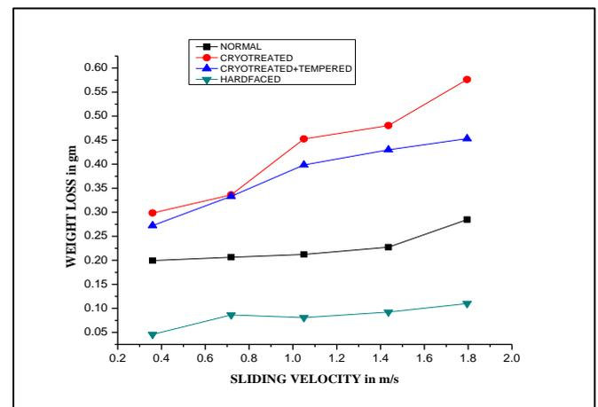
Fig. 5: (B) Graph of Weight Loss in Grams to Sliding Velocity in M/S
