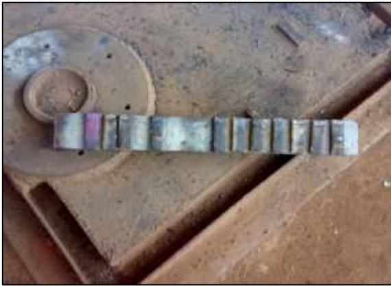
Fig. 2: Specimens Are Fixed On Iron Strip
