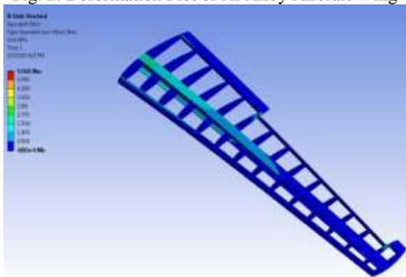
Fig. 3: Equivalent Stress Plot of Al Alloy Aircraft Wing
