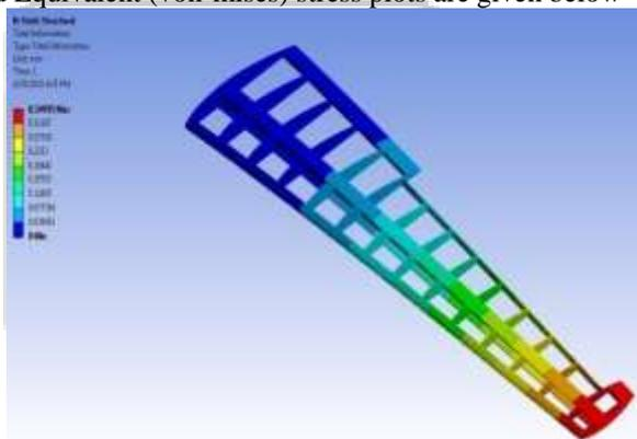
Fig. 2: Deformation Plot of Al Alloy Aircraft Wing
