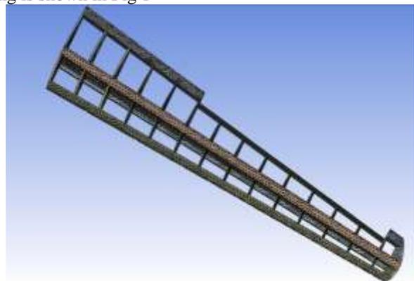
Fig. 1: Mesh Model of Aircraft Wing
