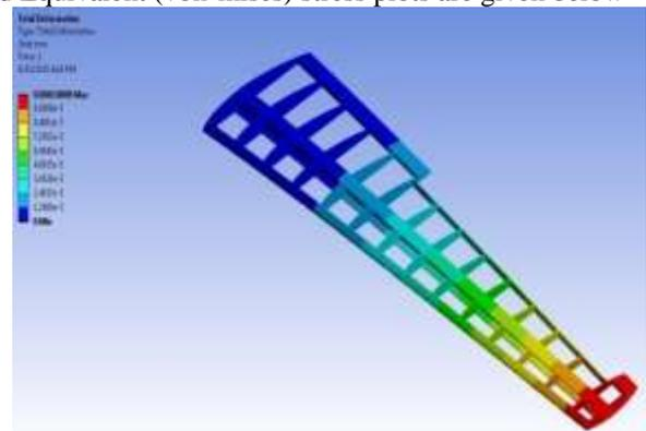
Fig. 4: Deformation Plot of Gr-Ep Composite Aircraft Wing
