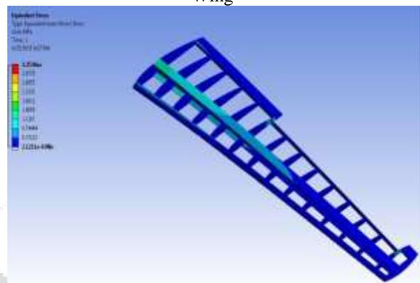
Fig. 5: Equivalent Stress Plot of Gr-Ep Composite Aircraft Wing.
