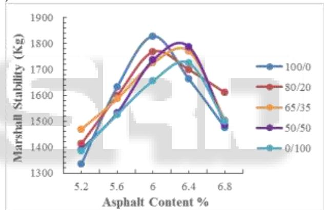
Fig. 2: Asphalt Content v/s Marshall Stability
