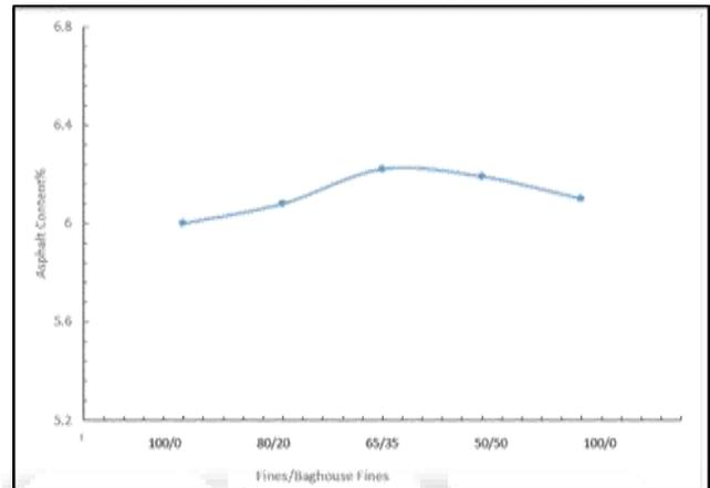
Fig. 7: Asphalt Content v/s F/BH Ratio
