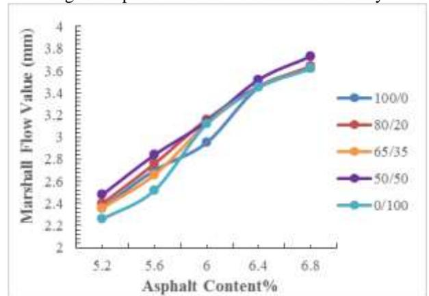
Fig. 3 Asphalt Content v/s Marshall Flow Values
