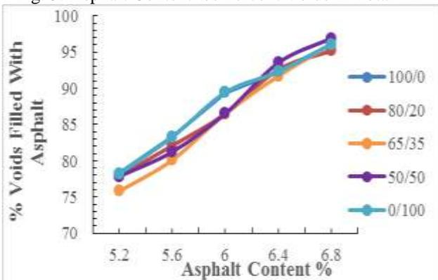
Fig. 6 Asphalt Content v/s Percent Voids Filled with Asphalt
