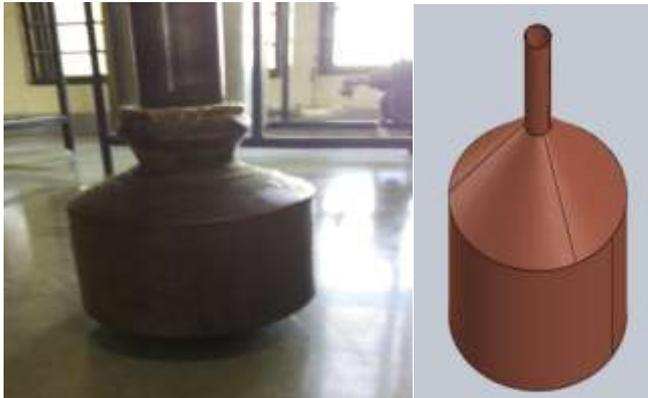
Fig. 1: displacer cylinder Actual and in designing Software
