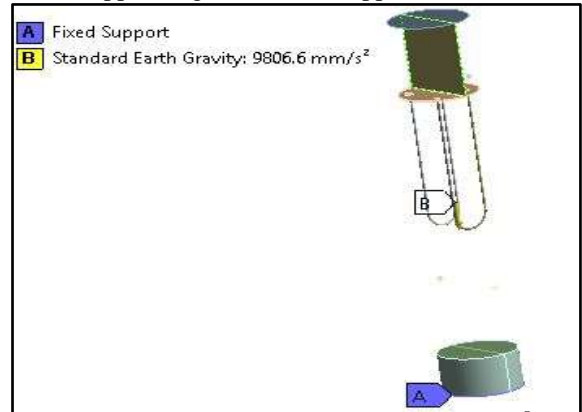
Fig. 5: self-weight boundary conditions
