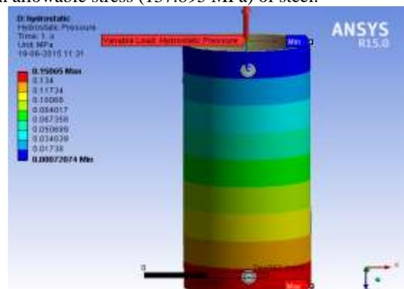
Fig. 6: Hydrostatic loading
