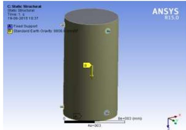
Fig. 4: self weight loading
