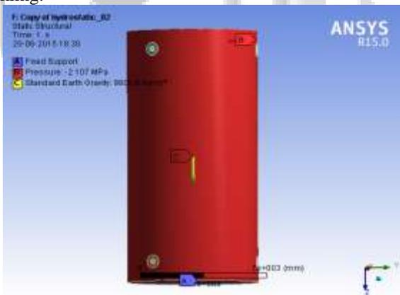
Fig. 8: Loading in linear buckling
