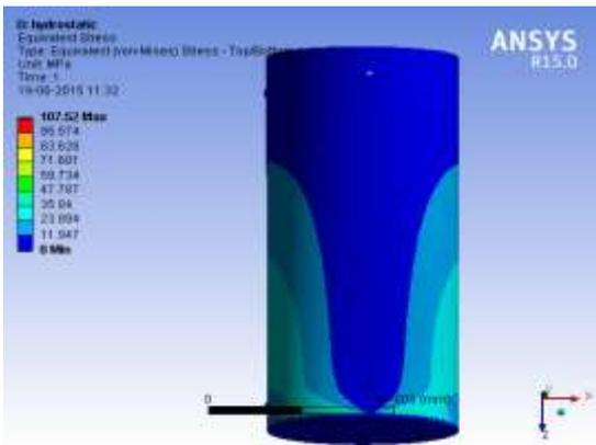
Fig. 7: Hydrostatic stress
