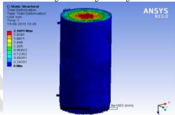
Fig. 5: Self weight deformation
