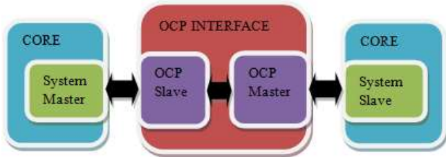
Fig. 2: Block Diagram of an OCP Interface
