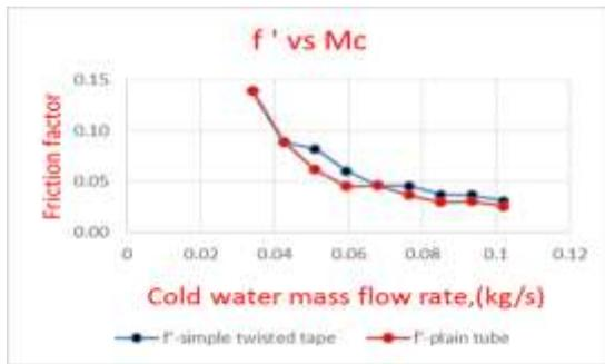
Fig. 4 Variation of friction factor with cold water mass flow rate for constant hot water mass flow rate for plain tube, simple twisted tape, modified twisted tape
