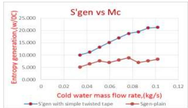
Fig. 7: Variation of Entropy generation rate with cold water mass flow rate for constant hot water mass flow rate for plain tube, simple twisted tape, modified twisted tape
