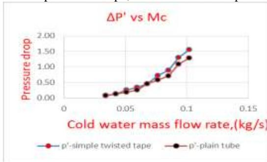
Fig. 5. Variation of pressure drop coefficient with cold water mass flow rate for constant hot water mass flow rate for plain tube, simple twisted tape, modified twisted tape
