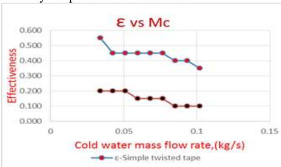
Fig. 6: Variation of Effectiveness with cold water mass flow rate for constant hot water mass flow rate for plain tube, simple twisted tape, modified twisted tape
