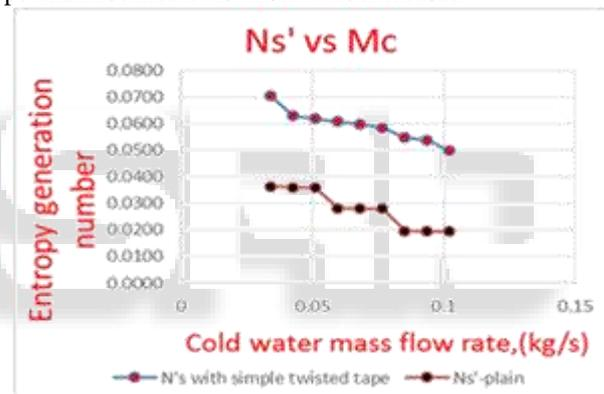
Fig. 8: Variation of Entropy generation number with cold water mass flow rate for constant hot water mass flow rate for plain tube, simple twisted tape, modified twisted tape
