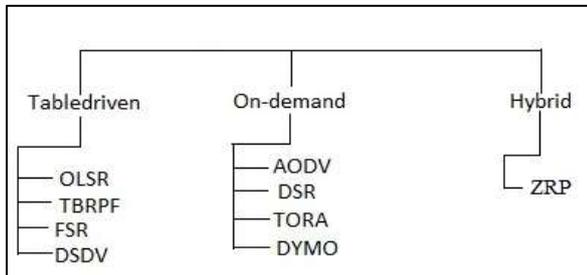
Fig. 2: Classification of Routing Protocols
