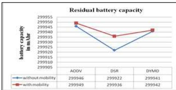
Fig. 8: Residual Battery Capacity of Traffic Nodes Per Protocol
