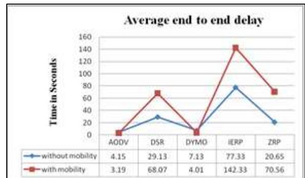
Fig. 10: Average End To End Delay Per Protocol In DEM
