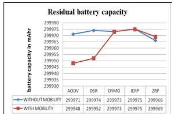
Fig.12: Residual Battery Capacity of Traffic Nodes per Protocol in DEM
