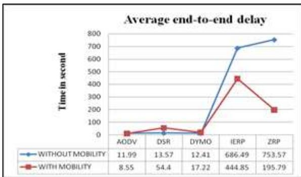
Fig. 6: Average End To End Delay Per Protocol
