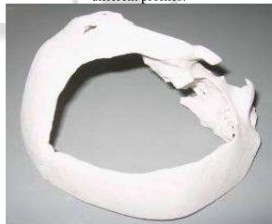
Fig. 9: A sliced 3D Z-Corp case study skull model.
