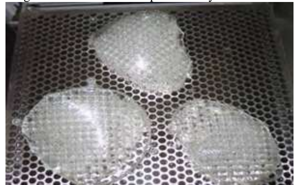
Fig. 10: Cranial plates rapid prototyped on 3D Systems 250 SLA machine
