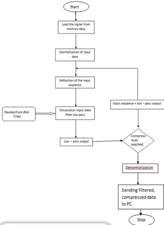
Fig. 2: Flow Chart of Discrete Wavelet Transform
