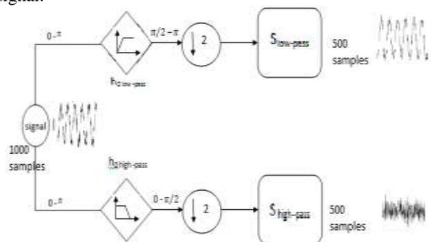
Fig. 1: Decomposition of Signal by the Pass Of The Signal Through Two Filters.
