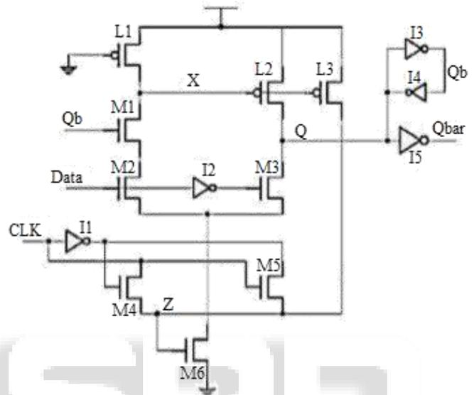
Fig. 2: Conditional pulse enhancement scheme FF [1]
