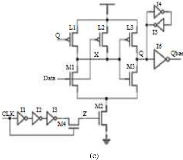
Fig. 1: Conventional pulse-triggered FF designs (a) ip-DCO (b) SCCER (c) MHLFF
