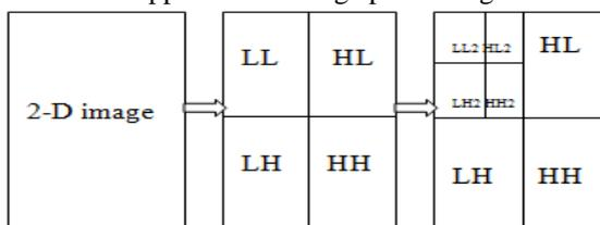
Fig 3.2: Wavelet Based Transform
