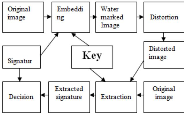
Fig. 1.1: Typical Watermarking block diagram
