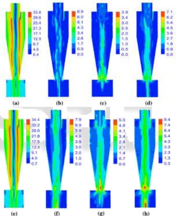
Fig. 6: Comparisons of RSTM and LES model from top to bottom and from left to right: mean velocity magnitude m/s, RSM tangential velocity m/s, RSM axial velocity m/s, and RSM velocity magnitude m/s. [3]
