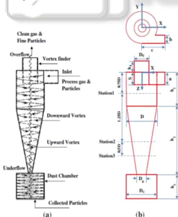
Fig. 4: Diagram of high efficiency stairmand cyclone geometry (a) working principle (b) Coordinate system for cyclone geometry. [3]
