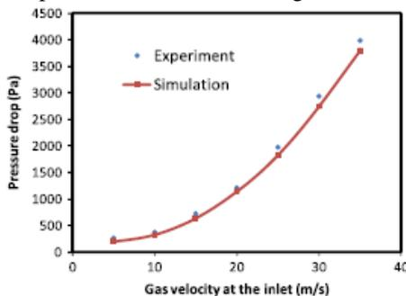
Fig. 13: Comparison of the simulated and measured pressure drops at different inlet gas velocities. [10]
