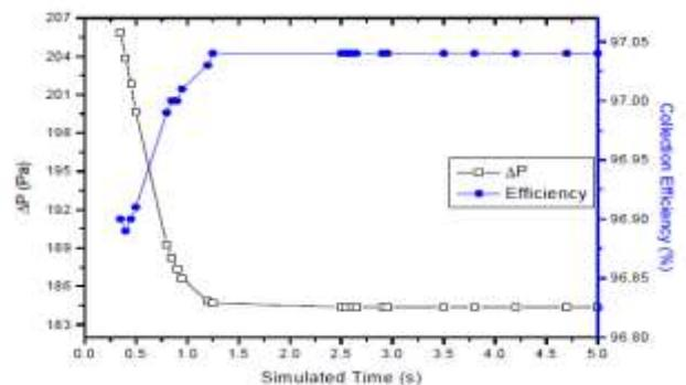
Fig. 3: Performance parameters profile cyclone with symmetrical inlet section using the LES model. [1]
