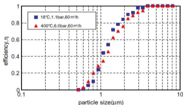
Fig. 9: The effect of temperature on the measured fraction collection efficiencies for 18 ° c and pressure drop 1bar and 6bar. [4]
