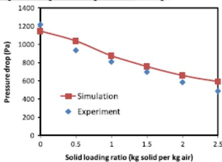
Fig. 12: Comparison of simulated and measured pressure drops at different solid loading ratios. [10]
