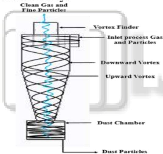
Fig. 1: Principle of cyclone separator
