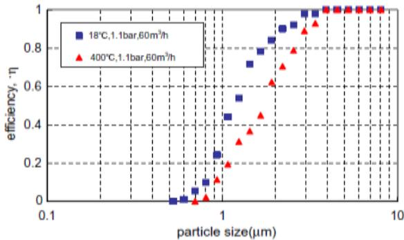
Fig. 7: The effect of temperature on the measured fraction collection efficiencies for 18 °c and 400 ° c temperature. [4]
