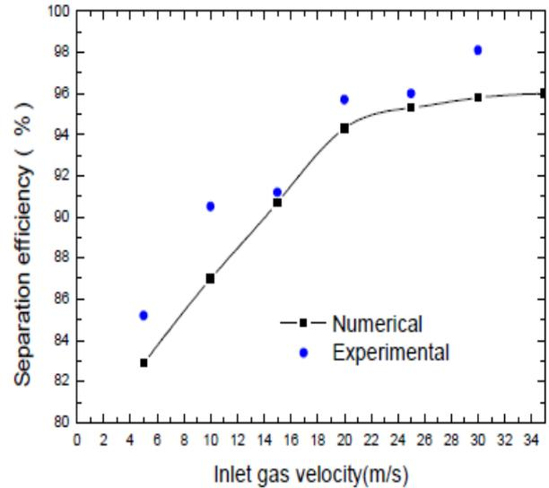
Fig. 13: Experimental results of separation efficiency compared with calculation results. [11]
