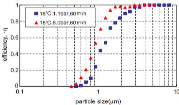
Fig. 8: The effect of temperature on the measured fraction collection efficiencies for 18 ° c and pressure drop 1bar and 6bar. [4]
