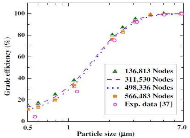
Fig. 5: Simulated grade efficiency profiles for the Stairmand cyclone of 0.3 m barrel diameter with different mesh density using RSTM technique. [3]
