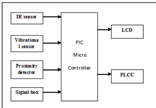
Fig. 1: Block Diagram of Proposed System Transmitter Module
