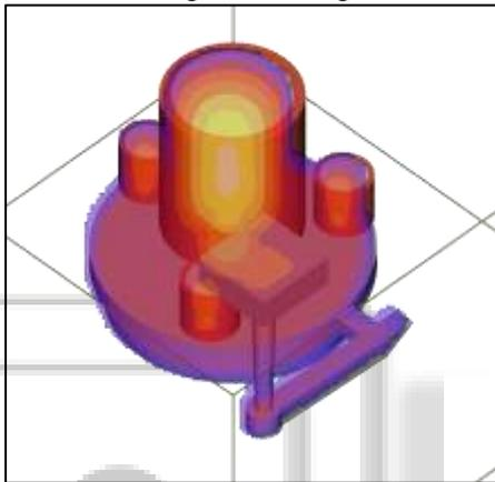
Fig. 6: Resimulation Result of The Part By Changing Gating Element Design
