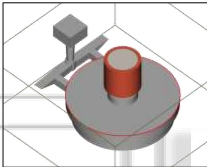
Fig. 3: Gating element design model input from Creo to the AutoCAST as STL format
