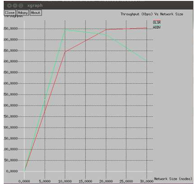
Fig 5: Comparison of Throughput in OLSR and AODV
