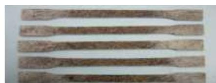
Fig. 1: Tensile test specimens
