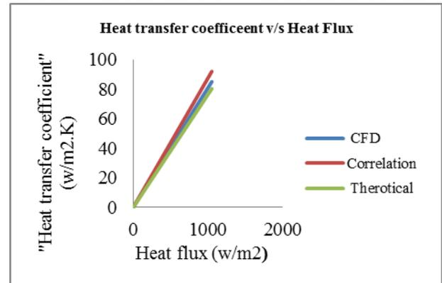
Fig. 10: Graph of Heat transfer coefficient v/s Heat Flux From the above figure it is clear that CFD value ( $85 \text{ w/m}^2\text{K}$ ) is nearer to the theoretical and correlations values (i.e.  $80.28$  and  $91.96 \text{ w/m}^2\text{K}$ ).
