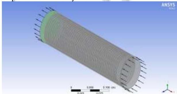
Fig. 8: Elliptical duct with thread inserted
