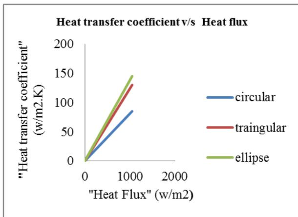
Fig.11: Graph of Heat transfer coefficient v/s Heat Flux of circular, triangular and ellipse
