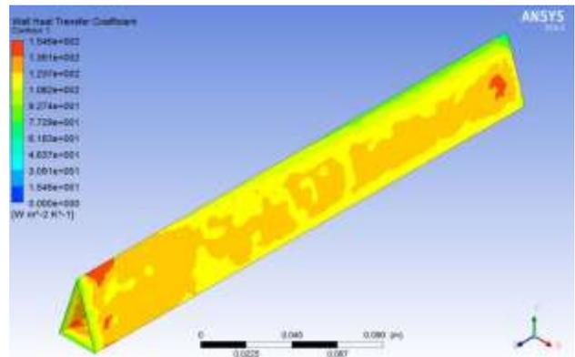
Fig. 4: Triangular duct with smooth surface
