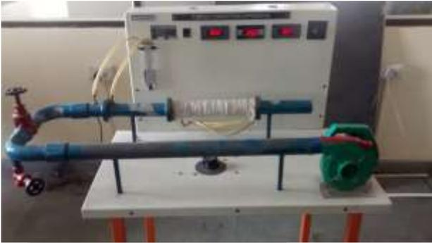
Fig. 1: Forced Convection Apparatus
