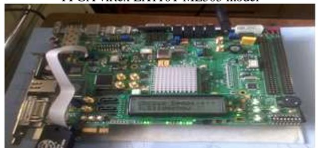
Fig. 5.6: Implementation after configuring the target device on FPGA Virtex5 XUPLX505T
