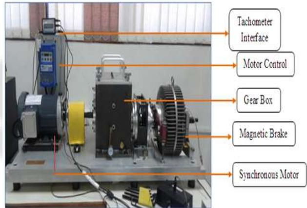
Fig. 3: Bearing Dynamics Simulator
