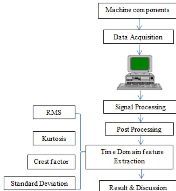
Fig. 4: Scheme of machinery fault diagnosis
