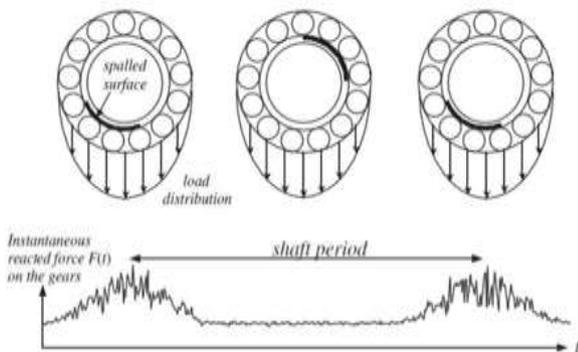
Fig. 2(B): Bearing Fault
