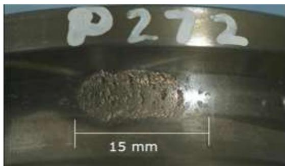
Fig. 8: Details of fault of bearing
