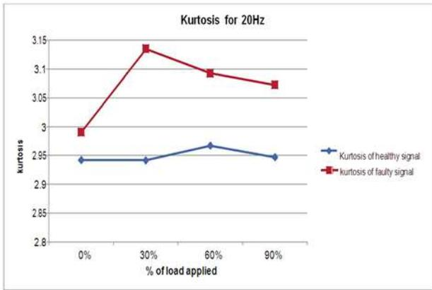
Fig. 15: Kurtosis comparison for different signals at 20Hz
