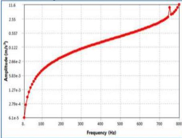
Fig. 11: ANSYS Acceleration Response (along Y axis) in Frequency Domain
