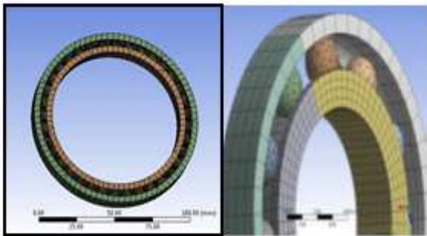
Fig. 6: Meshed model of bearing
