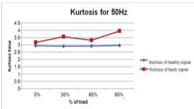
Fig. 16: Kurtosis comparison for different signals at 50Hz
