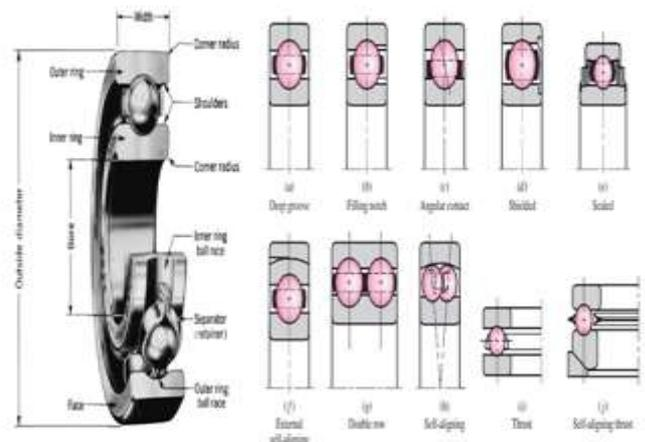
Fig. 1: Ball bearing & its types
