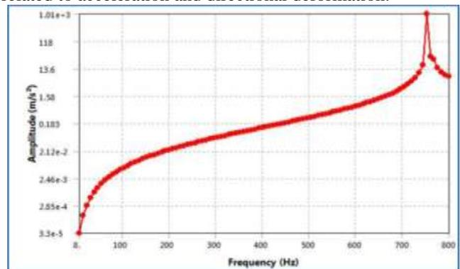
Fig. 10: ANSYS Acceleration Response (along X axis) in Frequency Domain
