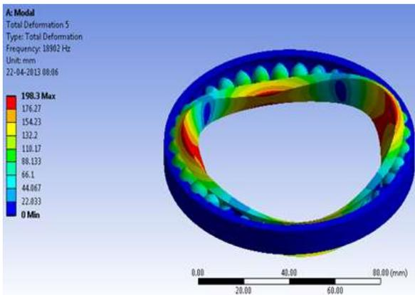
Fig. 7: Mode shapes of bearing without fault
