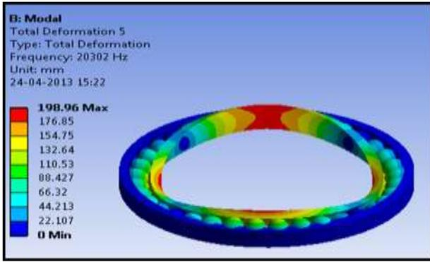
Fig. 9: Mode shapes of bearing with fault
