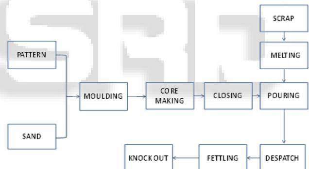
Fig. 1: Process flow diagram in a casting industry
