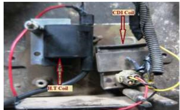
Fig. 5: CDI Coil & High Tension Coil
