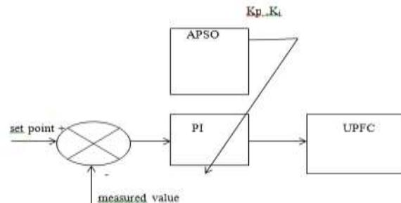
Fig 3: Optimal PI controller with APSO algorithm
