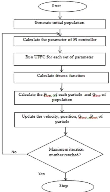
Fig: 4: The Flowchart of the PSO-PI Control System technique
