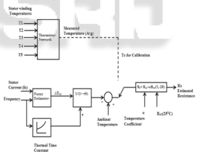
Fig. 3: Stator resistance estimator
