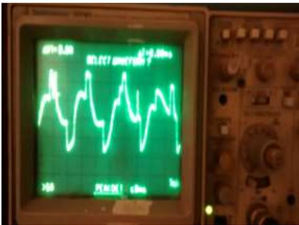
Fig. 7: Stator Current Waveform
