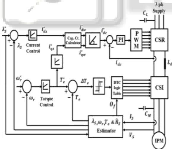
Fig. 2: Control strategy of CSI fed PMSM with DTC
