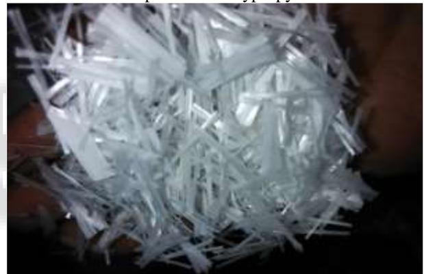
Fig. 1: Polypropylene Fibres
