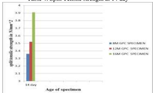
Fig. 2: Split Tensile strength at 14 day
