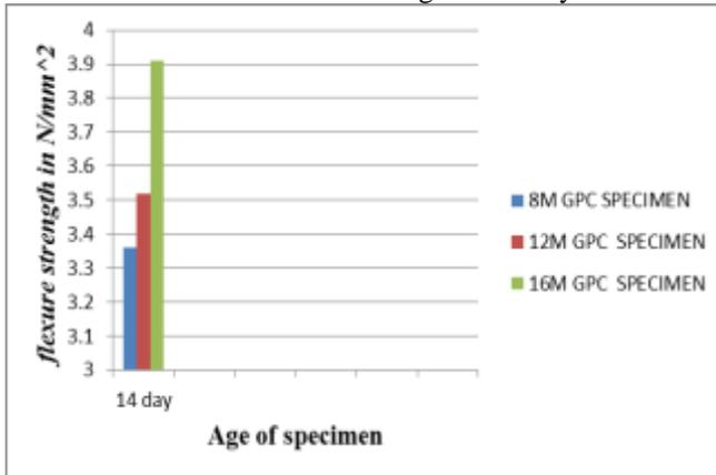
Fig. 3: Flexure strength at 14 day.
