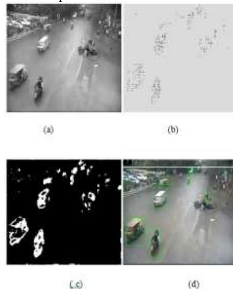
Fig. 3: An urban video frame (a) Gray-scale image, (b) optical flow motion vectors, (c) binary image with blobs and (d) tracking motion vehicles with boundary boxes.
