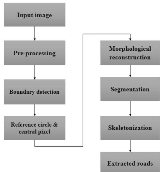
Fig. 1: Block diagram of proposed scheme
