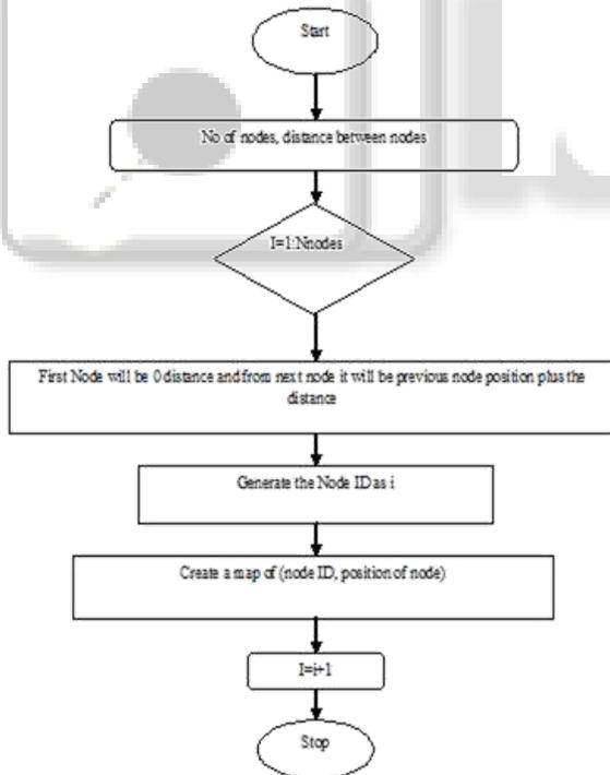
Fig. 1: Node deployment algorithm
