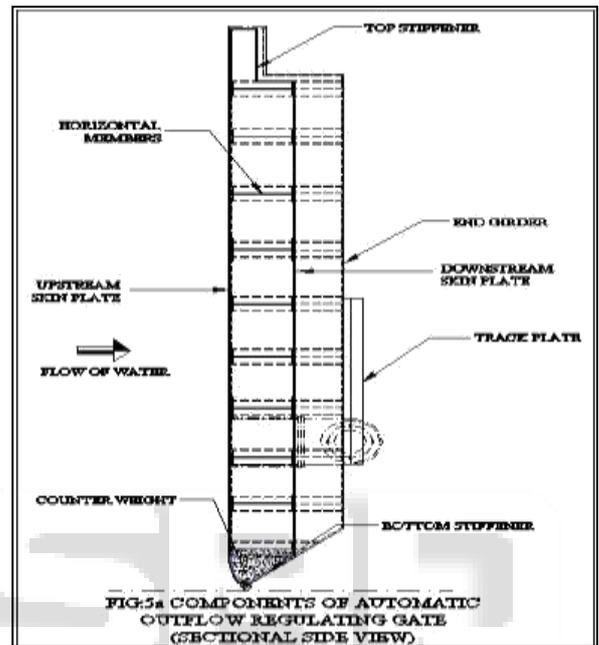
Fig. 5(a): Components of Automatic Outflow Regulating Gate (Sectional Side View)
