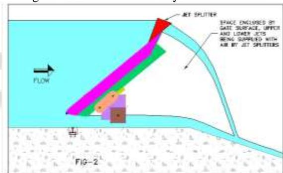
Fig. 2: Gate Stops to Move Further and Remains Stable in That Position
