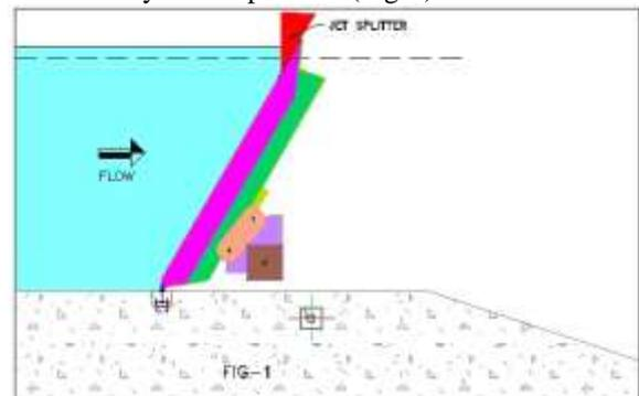
Fig. 1: Gate Remains in Fully Closed Position
