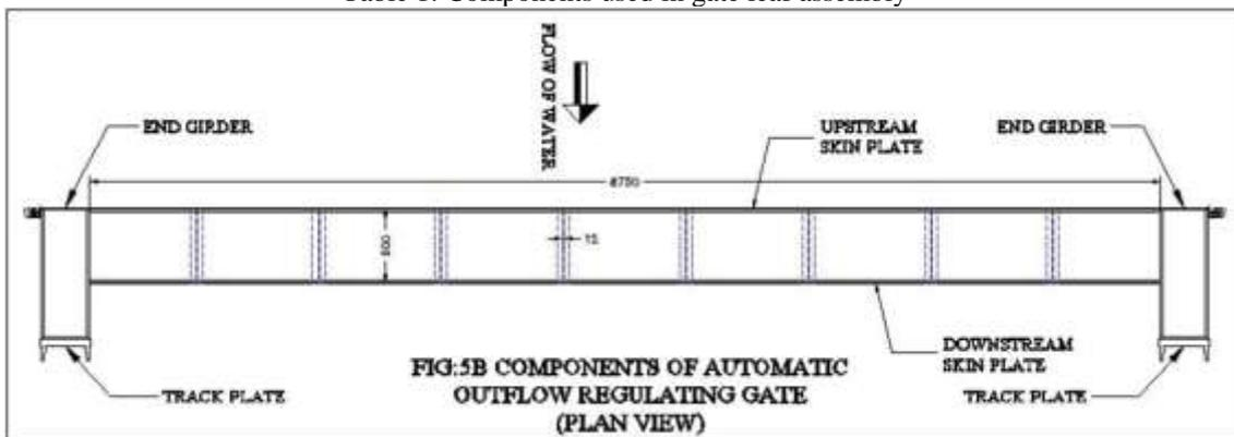
Fig 5(b): Components of Automatic Outflow Regulating Gate (Plan View)
