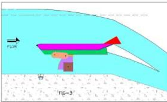
Fig. 3: Gate Opens out More & More until It Achieves Its Fully Open Position
