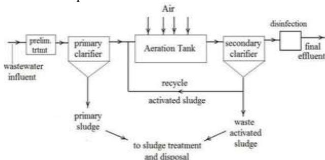
Fig. 2: Flow Diagram for Activated Sludge Process
