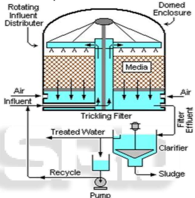
Fig. 3: Diagram of Trickling Filter
