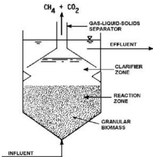
Fig. 4: Upflow Anaerobic Sludge Blanket
