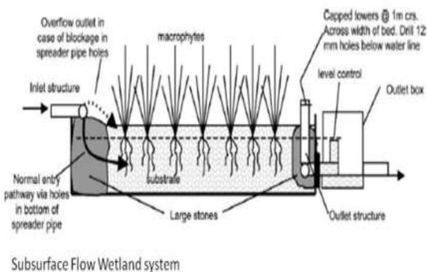
Fig. 5: Subsurface Flow Constructed Wetland
