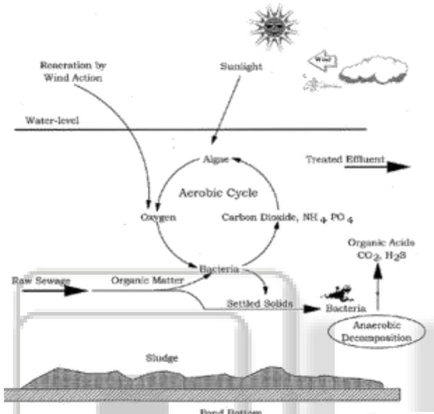
Fig. 1: Mechanism of Oxidation Pond
