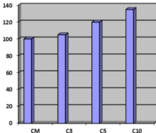
Fig. 1: Slump values for different mix proportions
