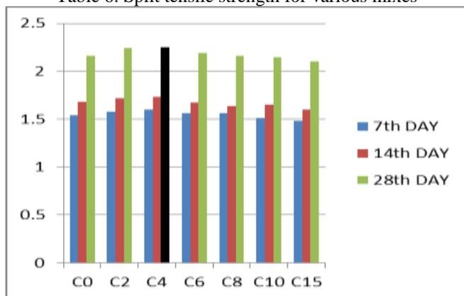
Fig. 7: Relation between split tensile strength of concrete and percentage clay
