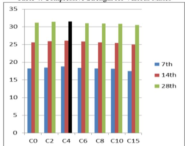
Fig. 2: Compression Strength Variation of Different Mix for 7, 14, & 28 Days
