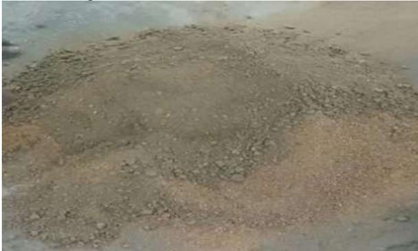
Fig. 1: Presence of clay in sand.
