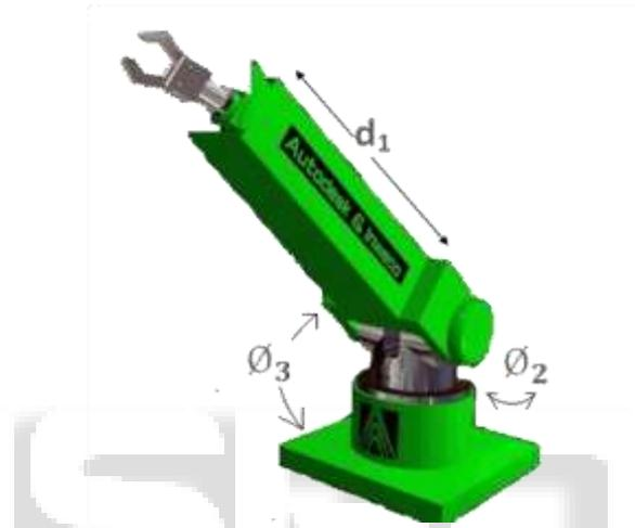
Fig. 1: Three Degree Freedom Robotic ARM
