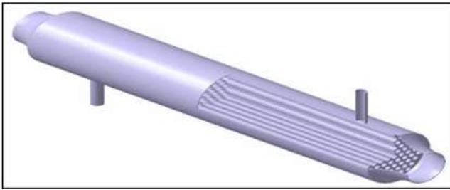
Fig. 4: EGR Cooler CAD Model
