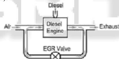
Fig. 1. Exhaust Gas Recirculation
