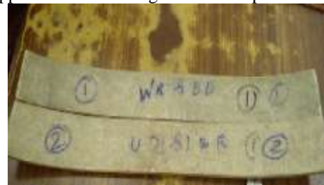
Fig. 4: The two leaf springs after fabrication. with dimensions 1. 350mm x 62.17mm x 10.1 mm 2. 350mm x 62.5mm x 9.1 mm (including the 1mm error)
