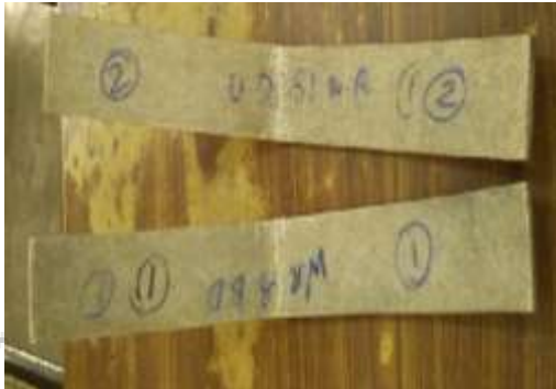
Fig. 8: The broken Specimens one and two after bending test
