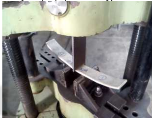
Fig. 5: The bending test performed in UTM for specimen one
