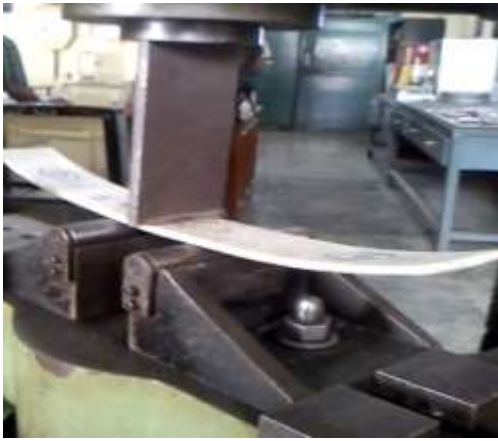
Fig. 7: The bending test performed in UTM for specimen two
