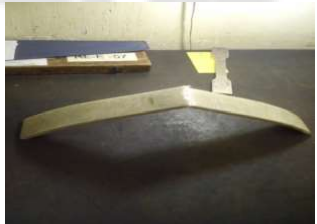
Fig. 6: The broken specimen one after bending test
