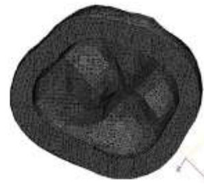
Fig. 10: Mesh Quality after Remeshing
