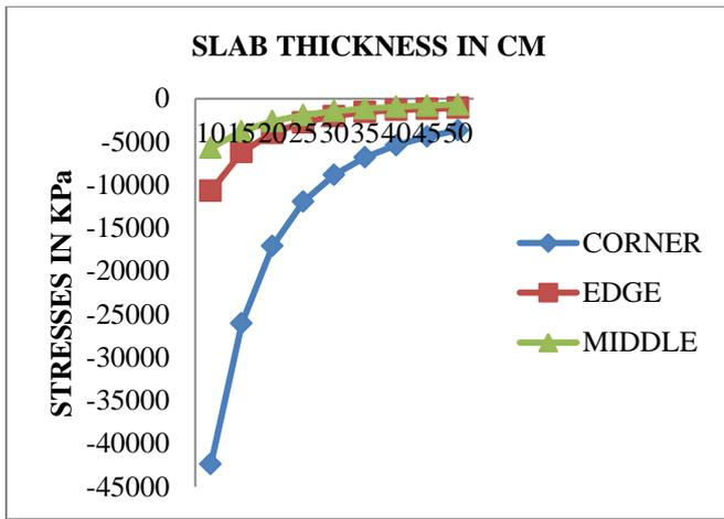
Fig.1: Thickness versus Stresses
