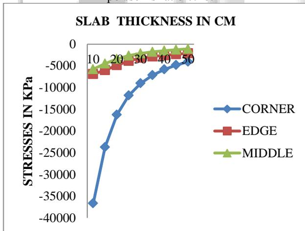
Fig.2: Thickness versus Stresses
