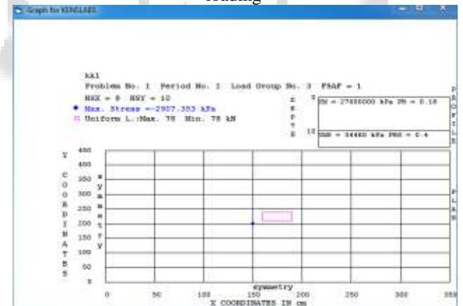
Fig.3: Rigid Pavement Model in KENPAVE for centre loading
