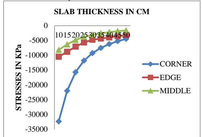
Fig.3: Thickness versus Stresses
