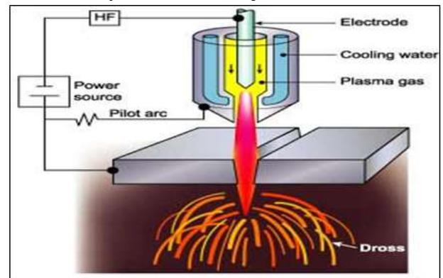
Fig. 1: Schematic diagram of plasma arc cutting
