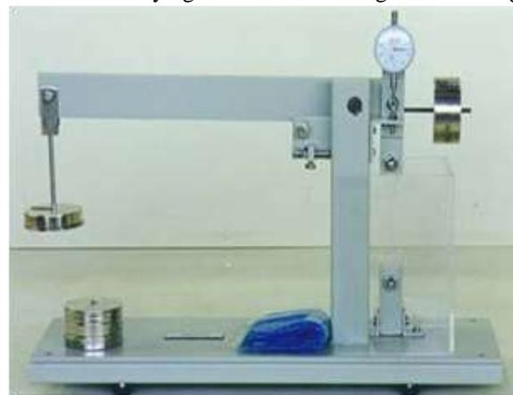
Fig.7: Creep testing machine
