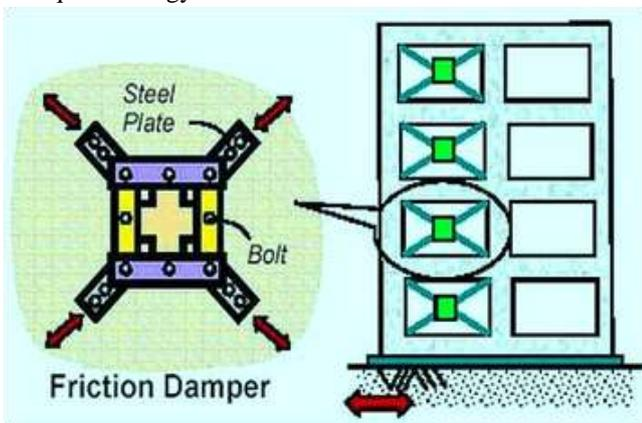
Fig.1: Friction damper that is used in multi-storey building
